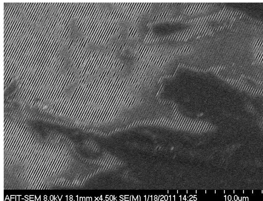
Fig 4.5 Large area capture of 230-nm S1805 features.
